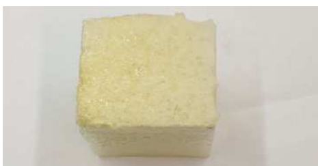
Figure 1. Citric acid/glycol foam with a density of 0.26 \text{ g}\cdot\text{cm}^{-3} (left) and solid cube from the same polymer mixture containing 20 wt% of recycled cellulose with a density of 0.89 \text{ g}\cdot\text{cm}^{-3} and a compressive strength of 23 \text{ N}\cdot\text{mm}^{-2} (right). Sample size 4 \times 4 \times 4 \text{ cm}^3 .
