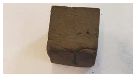
Figure 1. Citric acid/glycol foam with a density of 0.26 \text{ g}\cdot\text{cm}^{-3} (left) and solid cube from the same polymer mixture containing 20 wt% of recycled cellulose with a density of 0.89 \text{ g}\cdot\text{cm}^{-3} and a compressive strength of 23 \text{ N}\cdot\text{mm}^{-2} (right). Sample size 4 \times 4 \times 4 \text{ cm}^3 .
